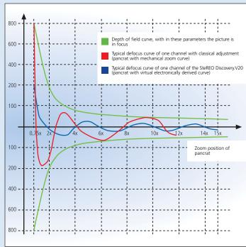
Illustration of the defocus curve of a classical mechanical pancrat in comparison to a motorized one (SteREO Discovery.V20). It is clear that the motorized pancrat differs from the 0 line about half less than the mechanical one. That means: SteREO Discovery.V20 with motorized pancrat delivers twice as sharp images.
