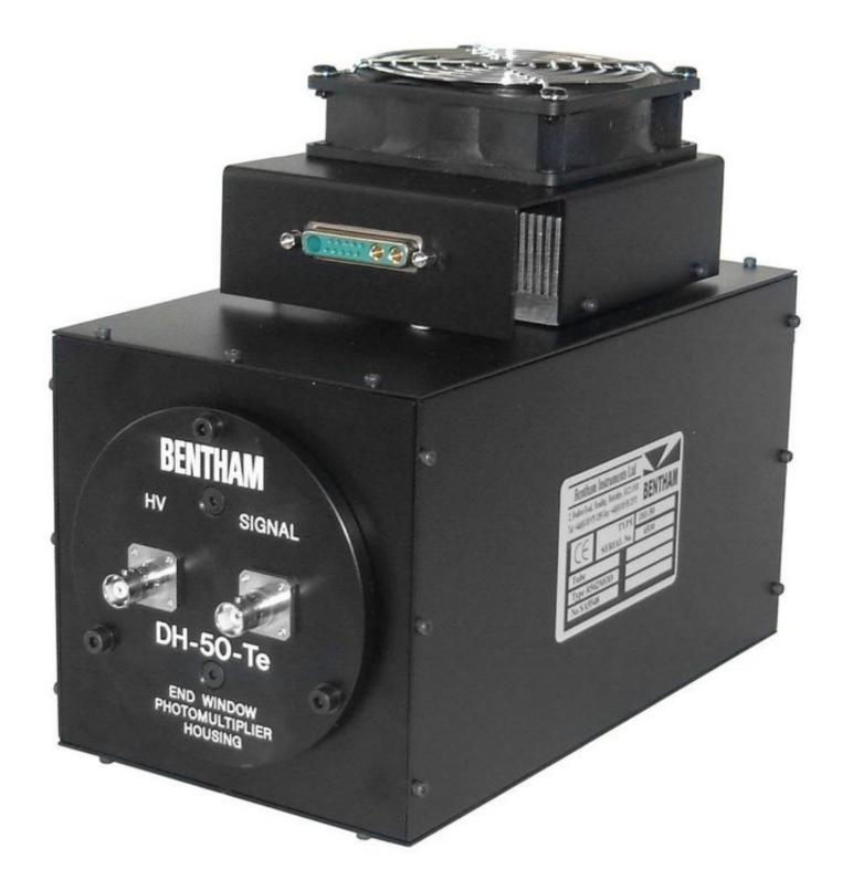
The DH\_50 photomultiplier uses temperature control to reduce dark current and extend spectral range of the S20 photocathode.
