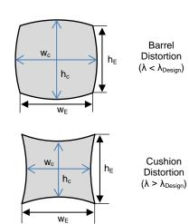
$\theta_{H}$ = horizontal angle,  $\theta_{V}$ = vertical angle,  $h_{C}$ = center height,  $w_{C}$ = center width,  $h_{E}$ = edge height,  $w_{E}$ = edge width
