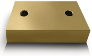
Fig. 3: The sub heatsink has to be attached to the bottom of the detector with a small amount of thermal epoxy. A thermally conductive adhesive tape can be an alternative. It is a flexible thermal interface from the detector to a larger heatsink, which has to be chosen and installed by the user.
