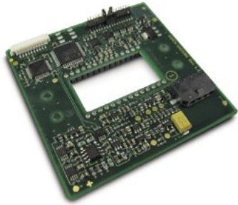
Fig 1: Backside of a sensor board PCB. There is a 28 pin socket at the top side that fits to the detector.
