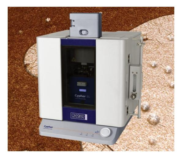
The Asylum Research Cypher ES builds on the exceptional performance of the Cypher S and adds full environmental control features. The same high resolution, speed and stability are maintained while easily operating in controlled gas or liquid environments, at temperatures from 0-250°C, and in some of the harshest chemical environments. The Cypher ES is the ultimate AFM for the most demanding experimental requirements.
