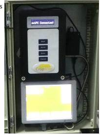
grain flows up the auger. The bin average shows the cumulative average for protein, oil and moisture since the START button was pushed to initiate the load. The protein, moisture and oil data can be stored in the CropScan 3000S' Touch Screen PC and later exported using a USB Memory Device or even through the internet directly to a remote PC.
