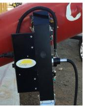
The **CropScan 3000S** is controlled and operated by a Touch Screen PC located in the cabinet. The data is displayed on the screen as a moving average and a bin average. The moving average shows the operator the protein, oil and moisture at approximately every 10 seconds as the
