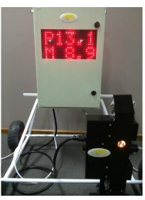
The bottom flap opens to release the grain and then closes ready for the next sample. The cycle time is approximately 7-11
