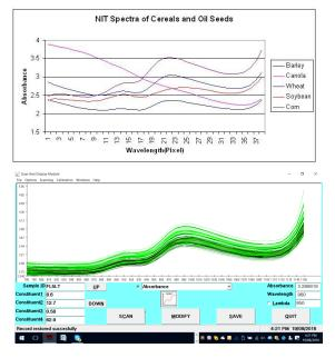
Calibration models have been developed to relate the amount of light absorbed by the sample to the concentration of each component. These calibrations are stored in memory and used to predict the protein, moisture and other components in samples of incoming grains and flour.
