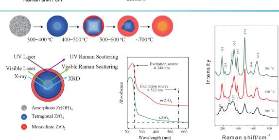
Raman spectroscopy can selectively obtain surface phase information of substances with strong absorption in the ultraviolet region (such as TiO<sub>2</sub> and ZrO<sub>2</sub>)
