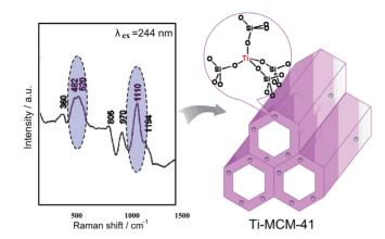
Microporous-ultra-low content of isolated transition metal ions in the framework of mesoporous materials (e.g.Ti-MCM-41) can be reliably and accurately identified by ultraviolet resonance Raman spectroscopy.
