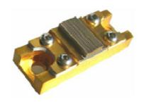
This stack "BS" type can be proposed with a variable number ('zz') of diode bars: 'zz' = 1 to 19 bars at a pitch of 400  $\mu$ m, 'zz' = 1 to 15 bars at a pitch of 500 μm 'zz' = 1 to 6 bars at a pitch of 1000 µm
