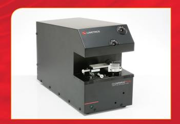
In 2015 Lumetrics was awarded a patent for an apparatus (now known as the ClearWave Plus) that measures the optical performance characteristics and dimensions of an optical element using a Shack-Hartmann wavefront sensor and a low coherence interferometer. This is a major improvement on current contact lens manufacturing inspection methods.
