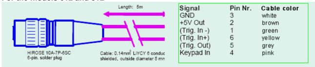
One end equipped with Hirose plug, the other with DB9; length 5 m
