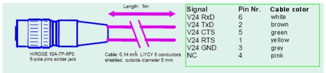
One end equipped with Hirose plug, length 5 m
