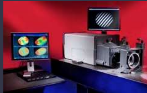
ZYGO GPI XP/D for measurement of cylindrical lenses
