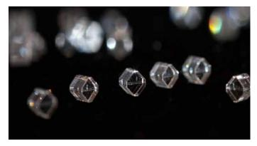
Single crystal CVD diamond prisms for use in spectroscopy applications.
