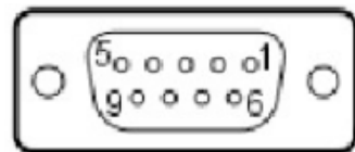
CORSIGHT PC system adapter cable, D-sub 9-pin connectors (RS-232)
