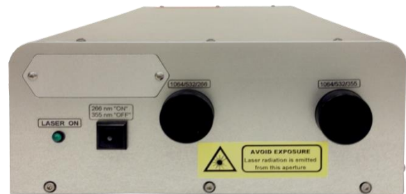
Laser with switchable 266/355 nm emission
