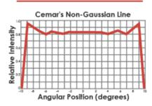
With Cemarline "Powershift™" the laser power is shifted slightly to the far end of the line delivering a clear balanced line from beginning to end.
