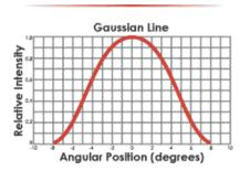
When angle mounted lasers use a fan lens to spread the light over the length of the line it loses intensity and fades out as it extends outward.
