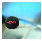
art photonics GmbH development of specialty fibers for the Mid-IR region has resulted in a unique product – Chalcogenide Infra-Red (CIR-) fibers. Chalcogenide glasses (As<sub>2</sub> S<sub>3</sub>) transmit IR-radiation in the spectral range of 1.1 – 6µm. Our CIR fibers are drawn in core/clad structure with double polymer coating and characterized by low total optical losses and low absorption peaks over mentioned spectral range.
