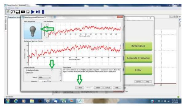
You will see a lot of noise until you **click the Strobe Enable** to turn the light back on. Then you should see the absorbance scale, with the trend near zero. If you left click on the graph a cursor appears and the wavelength and amplitude at that point are shown below the graph.
