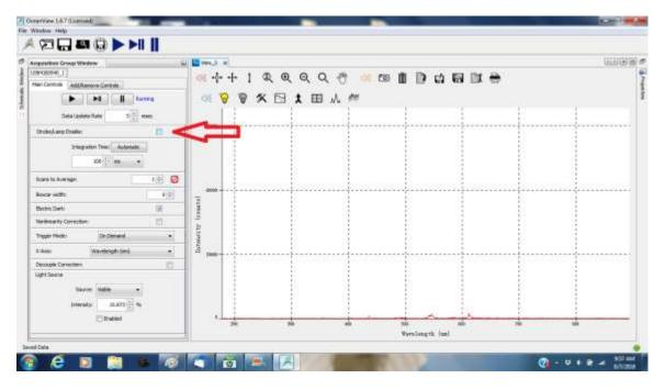
The default startup has the light source off (shutter closed) so the trace will be at the bottom. Check the Strobe Lamp enable button to turn the light on.
