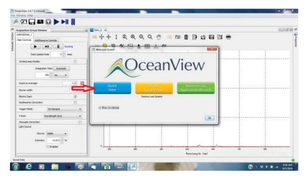
The startup text box appears, click on Quickview to check that the spectrometer is running, and to set up the control parameters in the Acquisition Group window.
