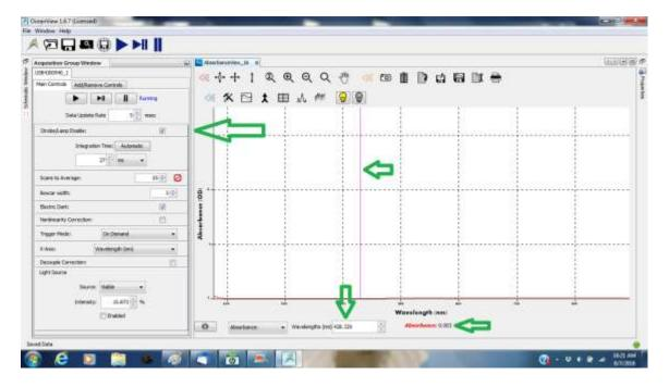
Now you are ready! **Put your sample in the cuvette well**. You will see the absorbance spectra displayed in real time. To see the absorbance at a single wavelength put the cursor on that wavelength and read the values below. The scroll bar on the wavelength text box lets you fine tune the cursor location.
