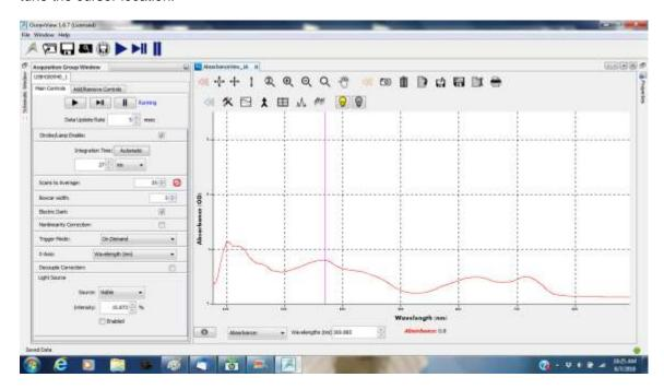
Icons have a hover message saying what they do. The camera captures the current spectra as an overlay. The sheet with a down arrow copies the spectral data to Windows clipboard.
