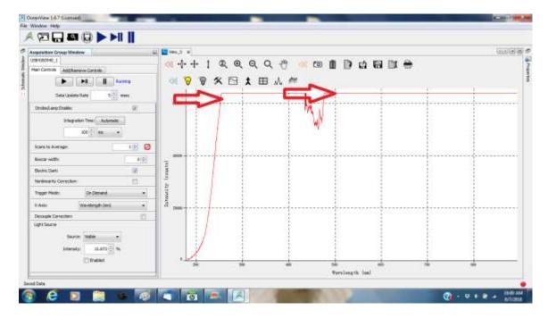
Now, adjust the sampling parameters in the Group acquisition box. The main control for sensitivity is the Integration Time (similar to the shutter speed on a camera). The default is 100 msec. To lower the signal, type in a shorter integration time. To get more signal make it longer.
