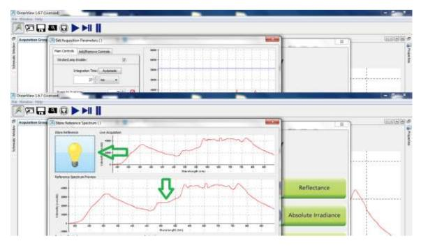
The lit light bulb icon will save the current spectra as the reference (blank). Each time you click it, software replaces the old values with the new values. The lower spectra shows what has been saved, the top panel shows the live trace. Click a few times to make sure the reading is stable, and is in fact showing the light source. The reference you are looking at is up to you. It can be air (nothing in the cuvette well) or a cuvette filled with the blank solution.
