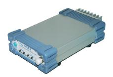
Safibra's SLEDs (Superluminiscent Light Emitting Diodes) are of Light Emitting Diodes (semiconductor light sources that merge the best features LEDs and semiconductor lasers. The SLEDs provide broadband output optical spectrum and low temporal coherence typical of LEDs, with high output power levels and high spatial coherence typical of semiconductor lasers.
