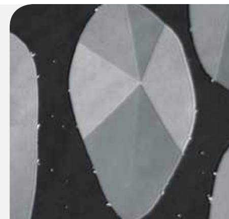
Monopalmitoyl-rac-glycerol at the air-water interface, surface pressure 4.22 mN/m
