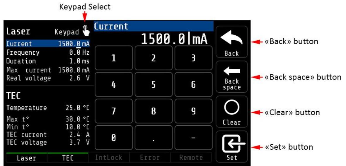
Fig. 11 – The *I Current Keypad* screen
