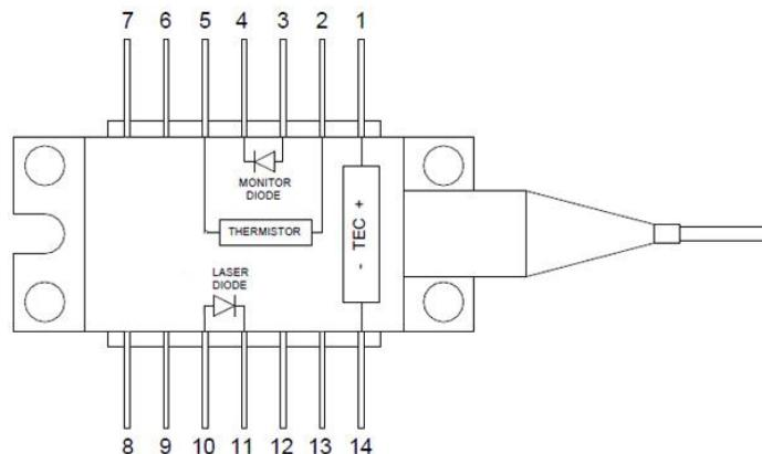
Fig. 5 – Pin functions type 1 Butterfly 14-pin
