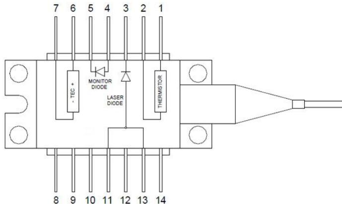
Fig. 6 – Pin functions type 2 Butterfly 14-pin
