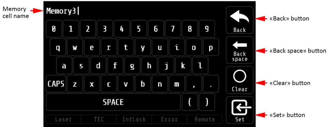
Fig. 17 -The *Memory Keypad* screen
