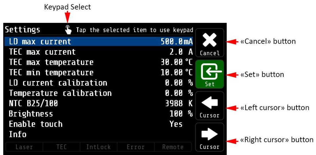
Fig. 15 – The Setting LD max current screen
