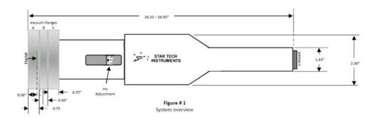
Model  $\mu$ BIP10x is a vacuum compatible (1x10-10 Torr) Beam profiler and Beam Imaging system designed for high resolution at 1-10 nm. The system is useful to 200 nm. The 10x mag. field of 1.5 mm has a resolution of 0.6  $\mu$ m and is sensitive to very low energy levels. The system has been designed for use with a 1.3 x 1.3" sensor but can be modified for other camera formats. Different magnifications and cameras are available upon request.
