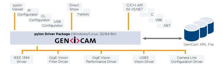
The internal architecture of the pylon driver package is based on GenlCam Technology, which offers you easy access to the newest camera models and the latest features. Changes to an existing camera device in your application essentially become a plug-and-play process.
