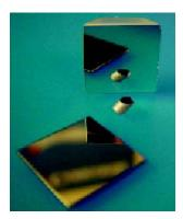
Mirrors have a highly polished surface for reflecting light. The reflecting surface is usually a thin coating of aluminum or silver. Most mirrors for optical applications are called first surface types since the coating is on the front surface thereby eliminating the optical properties of the glass from affecting the incident or reflected light. The rear surface is usually fine ground.
