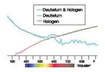
The AvaLight - DHc is both a deuterium light source and a halogen light source, providing you with adequate light between 200 and 2500nm for nearly all absorbance chemistry applications and more.
