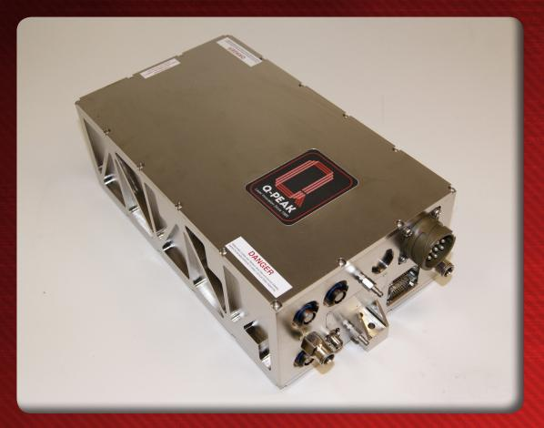
Q-Peak's Aurora 2520 laser provides a hardened laser architecture for highpower, high repetition-rate pulsed applications such as LADAR and mapping. Efficiently designed to minimize size, weight, and power consumption; Aurora utilizes a diode-pumped, solid-state laser architecture to conserve system resources while delivering high-energy, reliable illumination pulse streams.
