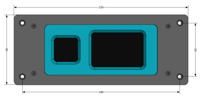
Figure 3-1: Dimensions for in-wall mounting with cover panel
