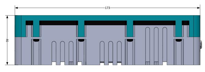
Figure 3-5: Side view without cover panel
