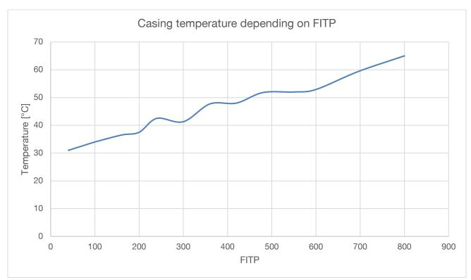
Figure 6-2: Expected cooling plate temperature depending on frame-rate integration time product
