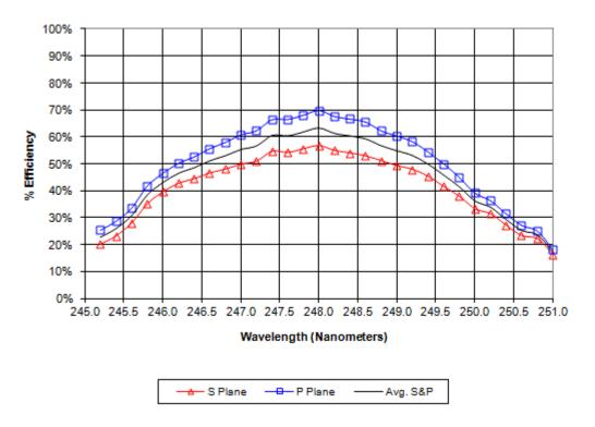
**Note:** The efficiency curve above is absolute and was measured in an in-plane near Littrow configuration (unless otherwise indicated). Efficiency curves are only representative: actual efficiency may vary significantly depending on use geometry and measurement technique. This efficiency curve is for master MR226; two masters with the same catalog number may have different efficiency curves. The uncertainty band on the data in the above efficiency curve(s) is +/- three percentage points.
