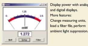
Display power with analog and digital displays. More features: Change measuring units, load a filter file, perform
