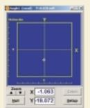
Real Time display of X,Y beam angle. features: Set relative center.
