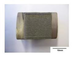
Using laser dispersion, metal-ceramic coatings can, for example, be added to moulding tools. These coating improve both the wear and corrosion characteristics of the tools, and can thus increase tool life.
