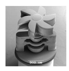
In the field of job order production, the Laser Zentrum Hannover e.V. (LZH) manufactures micro-components made of liquid, light-curable plastics or carries out feasibility studies.
