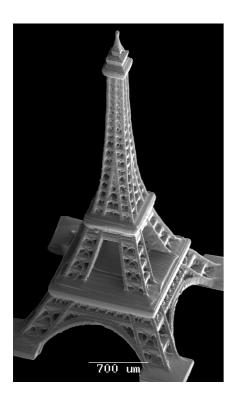
The LZH offers consulting, feasibility studies and process development for the additive manufacturing of polymer parts. With micro stereo lithography, 3D parts can be manufactured with a resolution of > 5  $\mu m$ . An aerosol jet process enables multi-material manufacturing processes on uneven surfaces, too.
