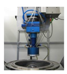
With the application of material by laser cladding, components can both be protected from wear or repaired.
