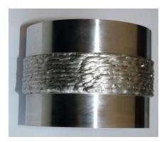
During laser-assisted arc deposition welding, the laser beam stabilizes and guides the electrical arc. Thus, low dilution rates (<5%) and a precise positioning of the deposition material can be achieved.
