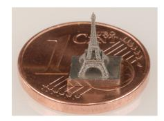
Additive manufacturing processes can be used to manufacture highly precise and complex workpieces.
