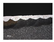
Using laser alloying, wear-resistant coatings can be placed on different materials. For example, materials with a high carbon affinity can be embedded in the surface of a basis material. These embedded materials react with the carbon in the basis material, forming wear-resistant carbides.
