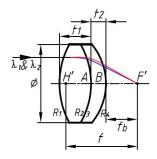
Achromatic lenses are very common type of viewer lenses, they consist of two or more lens elements, which have been corrected for chromatic aberration with respect to two selected wavelengths, The elements must be fixed in relation to one another by either mounting or cement.
