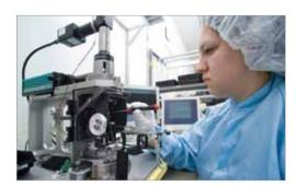
The zoom body adjustment device calculates the zoom control curve from around 7,000 reference points.
