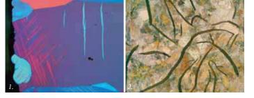
1. Zinc with deformation twins, 200x magnification, polarized light
