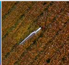
Laser-crystallized silicon on glass, EC EPIPLAN 10x/0.3
