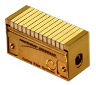
The H Package laser diode array is designed specifically for direct diode applications (e.g. hair removal and plastic welding). The package is offered in two dimensional configurations and is operational from 0.5ms to 300ms long pulse durations at up to 150 Watts per bar operation. The standard package is offered in <u>8-bar</u>, <u>10-bar</u> and 12-bar vertical stacks (custom options available upon request).
