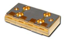
The AAAA package is a compact, conductively-cooled laser diode array. The AAAA package is available in pulsed configurations with up to 9.6 kW of peak power or in CW configurations with up to 160 W of continuous power.
