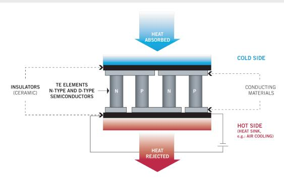
FIG. 1. Schematic of a thermoelectric device where the Peltier effect is used to generate heat flow between two materials.
