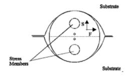
Evanescent wave couplers offer inherent performance advantages because there is no deformation or tapering of the waveguiding cores. These devices have low loss and backreflection. Also, short interaction lengths (1-2 mm) allow small device packages to be realized.
