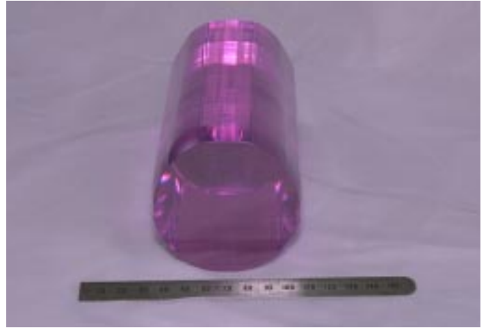
Ø75 x 208 mm boule section (Nd:YAG, 1.1 atom % Nd concentration)
