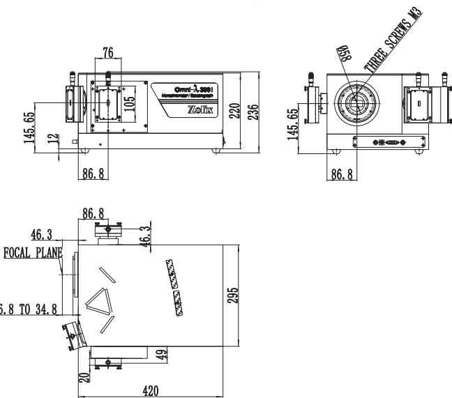
Omni- $\lambda$ 500i Monochromator/Spectrograph
