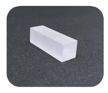
Due to the high damage threshold, wide transparency range LBO — Lithium triborate crystals are mostly used for second harmonic generation (SHG) a.k.a. frequency doubling and third harmonic generation (THG). Crystals can be heated up for protection or performance stabilization and then they can be used in high power applications.
