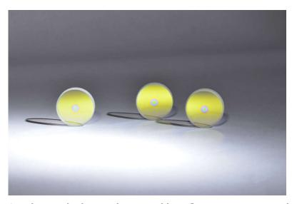
Variable reflectivity mirrors (VRM) also known as Radial Gradient Reflection Mirrors (RGRM), Graded Reflectivity Mirrors (GRM) or (Super) Gaussian Mirrors are unique optical mirrors designed for specific wavelength with reflection value variation as a function of radius (position form the center of mirror on the mirror 's surface). Usually – the highest reflectivity in the center. These mirrors can be produced only by few optical thin film coating companies worldwide.
