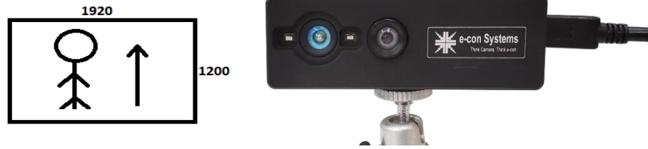
Figure 9: Camera Image Orientation with respect to USB Cable
