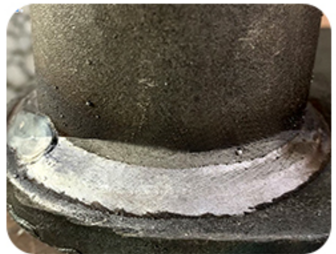
Weld Seam Cleaning
