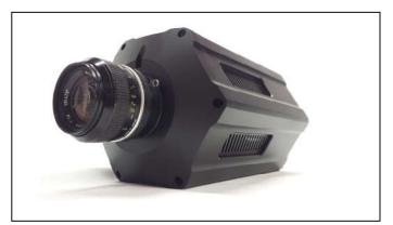
This lattice matched InGaAs camera allows for high resolution SWIR imaging 1280x1024 at high frame rates >93 frames per second (fps) at full frame size. This small pitch array, 12  $\mu$ m, combined with the high quantum efficiency of the lattice matched InGaAs arrays enables impressive imaging in the SWIR and visible band. The camera has the capability of four setpoints, 20°C (no cooling), 0°C (fan cooling), -40°C, or -60°C (water cooled) using a 3 stage TEC integrated in a vacuum package.
