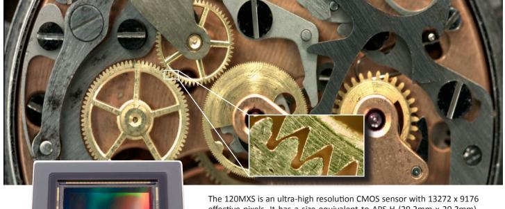
effective pixels. It has a size equivalent to APS-H (29.2mm x 20.2mm), and a square pixel arrangement of  $2.2\mu m$  x  $2.2\mu m$  with 122 million effective pixels. Ultra-high-resolution is made possible by parallel signal processing, which reads signals at high speed from multiple pixels. All pixel progressive reading of 9.4 fps is made possible by 28 digital signal output channels. It is available in RGB, RGB-NIR, or in monochrome with twice the sensitivity.
