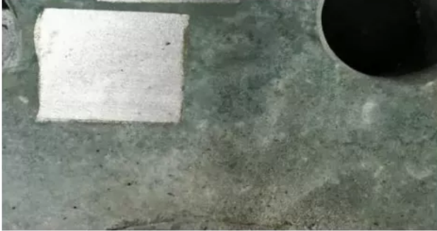
Cleaning the verdigris on copper alloy surface
