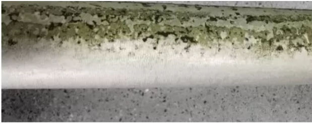
Cleaning the oxides and pollutants on steel tubes surface
