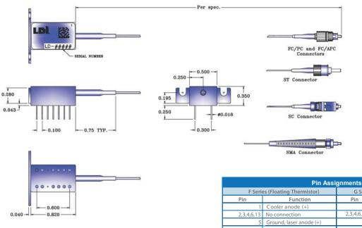
G Series (Ground Thermistor) Pin Function Cooler anode (+) No connection Ground, laser anode (+) Detector cathode (-) Detector cathode (-) 8 Detector anode (+) Detector anode (+) 9 Laser cathode (-) Laser cathode (-) 10 Ground Ground, thermistor 10 Thermistor Thermistor 14 Cooler cathode (-) Cooler cathode (-) 14
