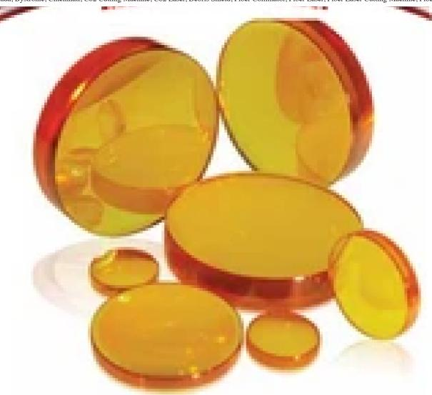
141972 - Focus Lens. Dia 1.5" (38.1mm) FL 9.0" (228.6mm) ET .291" (7.4mm) Meniscus ZnSe Suitable to be used with Trumpf(R) Laser System
