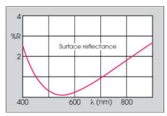
Two typical curves are shown for each coating. Curve 2 applies only to convex surfaces of short radius (R greater than 1.33 x dia.) and Curve 1 to all other surfaces.
